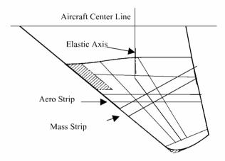
$Fig. \ 11 \quad F\text{-}15 \ stabilator \ modeling \ issues \ for \ doublet \ lattice.$
