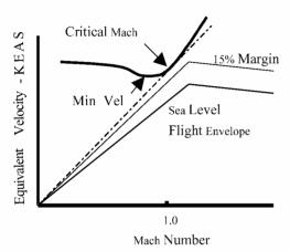
Fig. 15 Flight envelope and flutter boundary.
