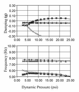
Fig. 21 Nonlinear flutter results obtained using ZTAIC.
