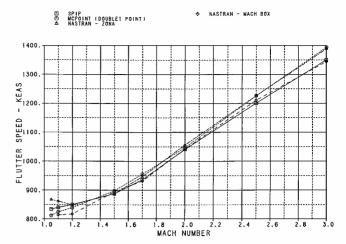
Fig. 6 Flutter speeds predicted by four supersonic aerodynamic codes.
