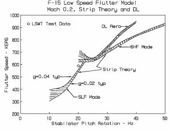
Fig. 10 Flutter speed predicted using doublet lattice and experimental data for the F-15 stabilator.
