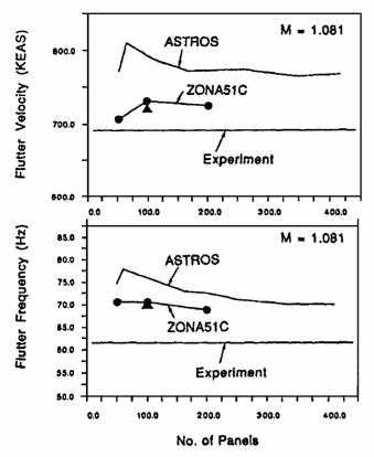
Fig. 4 Effects of panel numbers on flutter speed and frequency.
