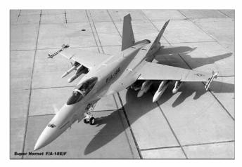
Fig. 16 Typical high-performance military aircraft with external stores.
