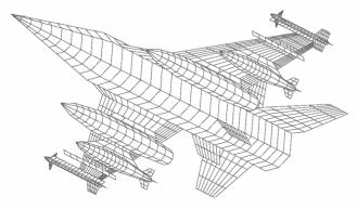
Fig. 19 ZONA code ability to model fighter-type aircraft with external stores.
