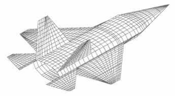
Fig. 18  $\,$  Modeling capability for ZONA code demonstrated for generic fighter aircraft.
