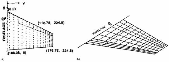
Fig. 1 Aerodynamic modeling of F-18 wing.
