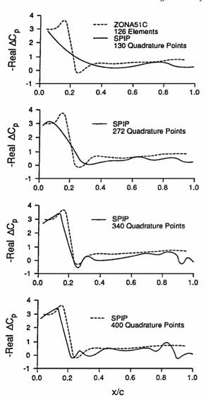
Fig. 2 Effect of panels on computed pressures for an F-18 wing with an oscillating leading-edge flap at 58.8% span, M = 1.1 and k = 4.0.
