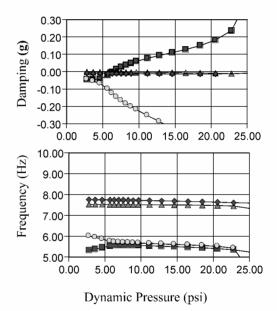
Fig. 20 Linear flutter results obtained using ZONA6 for Mach 0.9.
