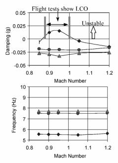
Fig. 22 Damping and frequency vs Mach number for LCO calculation based on ZTAIC: ♠, mode 5; ♠, mode 7; and ♠, mode 8.
