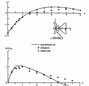
Fig. 5 Real and imaginary part of the lift on the main wing due to pitch of the canard, M = 1.054.
