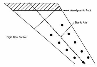
Fig. 3 U.S. Air Force Wright Aeronautical Laboratories. AFWAL wing flutter model with lumped mass NASTRAN representations: ●, structure grid points and ●, lumped masses.
