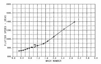
Fig. 7 Predicted flutter speed matchup with doublet lattice for two supersonic aerodynamics codes:  $\Box$ , MSC (subsonic);  $\bigcirc$ , MSC (supersonic);  $\triangle$ , MCPoint (subsonic); and  $\diamond$ , MCPoint (supersonic).
